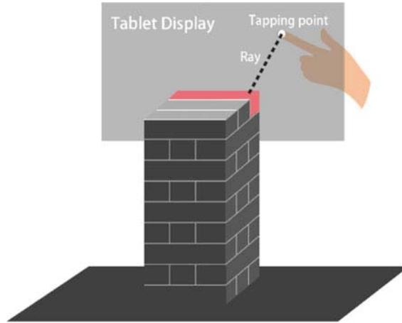
**Fig. 6** The ray casting technique implemented in mobile tablets. Touching a block to enable selection
