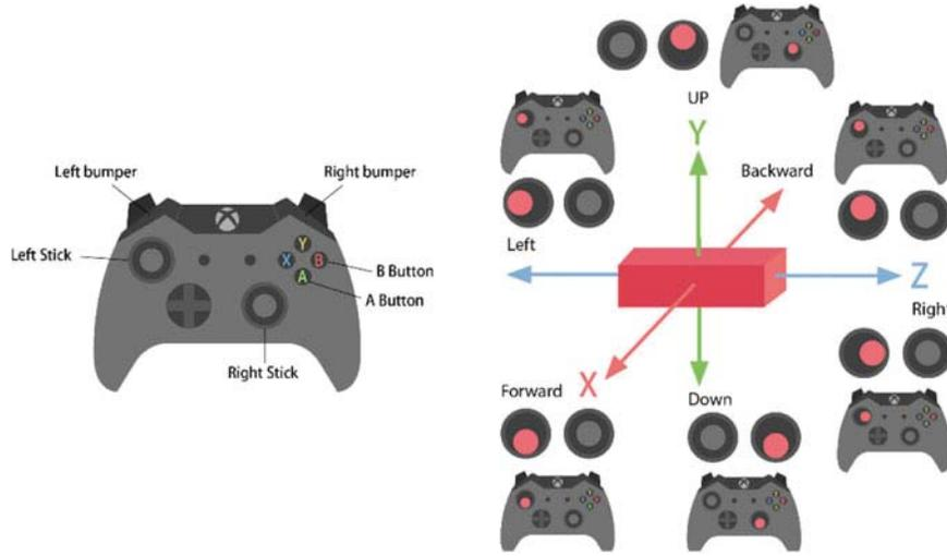
**Fig. 4** (Left) A typical modern game controller; (Right) How to move the selected block along the X, Y, Z axes
